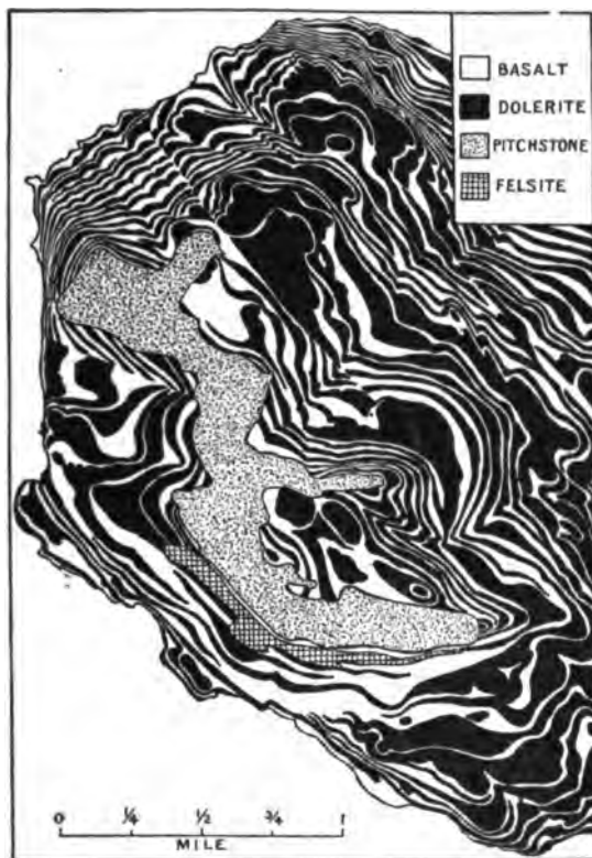
FIG. 2.—Dolerite sills cutting basalts, Isle of Eigg. (After A. Harker, Quart. Jour. Geol. Soc., Vol. 62, 1906, p. 44.)
